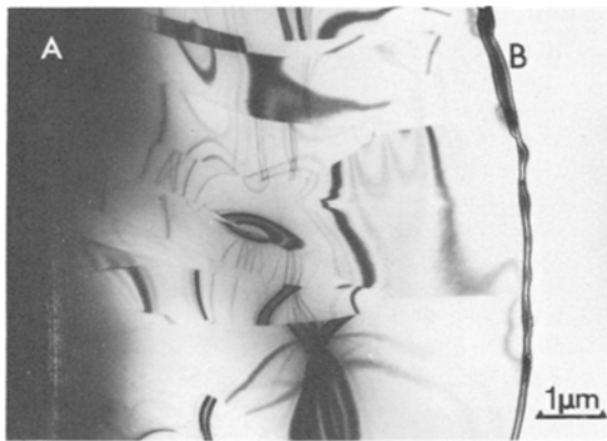
Figure 2 An electron transparent region produced by single droplet spreading in a splat quenched Al-17.3 at.% Cu alloy.
